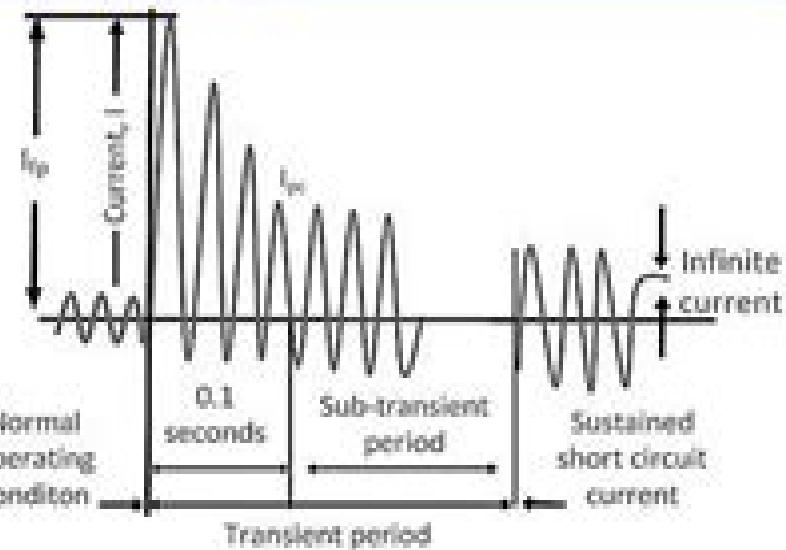
When two or more conductors of different phases come in contact with each other in a power line, power transformer or any other power element, then the part of the impedance is shunted out of the circuit due to which a large current flow in the un-faulted phases, such current is called the short circuit current. Short circuit current reduces the effect of impedance in the circuit while the current in the circuit rises.
