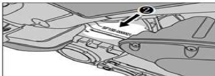
The frame serial number ① is stamped on the right side of frame under the footboard.
