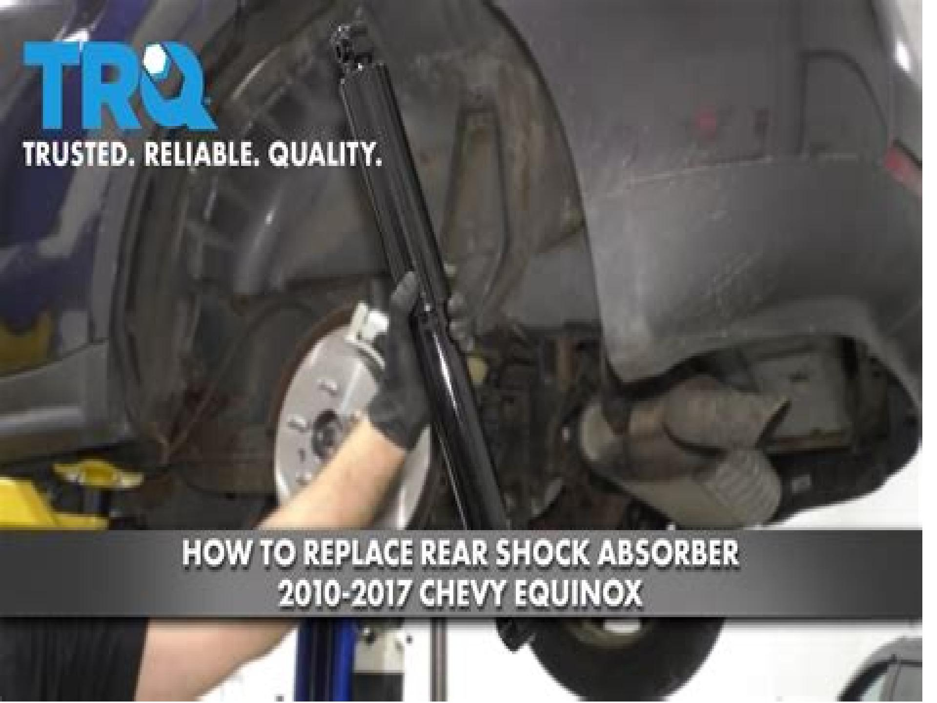
A close-up, slightly blurred photograph of a car's rear suspension system. The focus is on the shock absorber, which is a vertical cylindrical component. The surrounding area includes the wheel well, a coil spring, and various metal brackets and bolts. The background is dark and out of focus.
