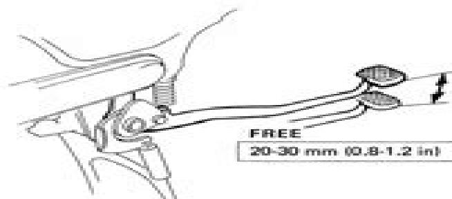
Adjust rear brake pedal free play by turning the adjusting nut which is located at the rear wheel.
