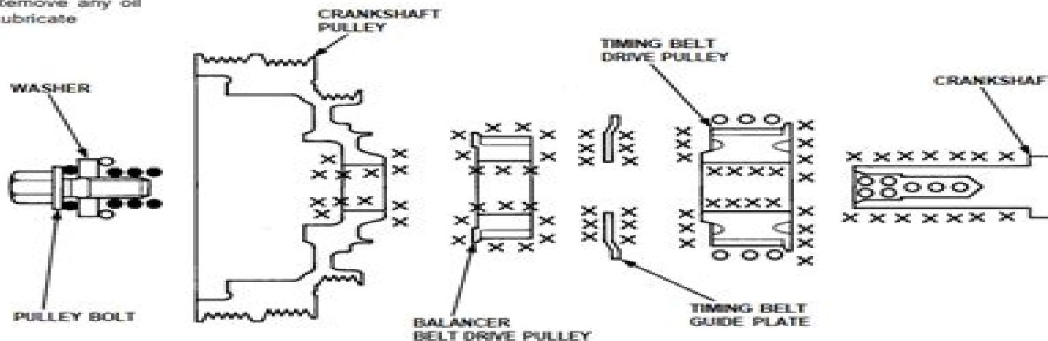
Crankshaft pulley bolt size and torque value:
