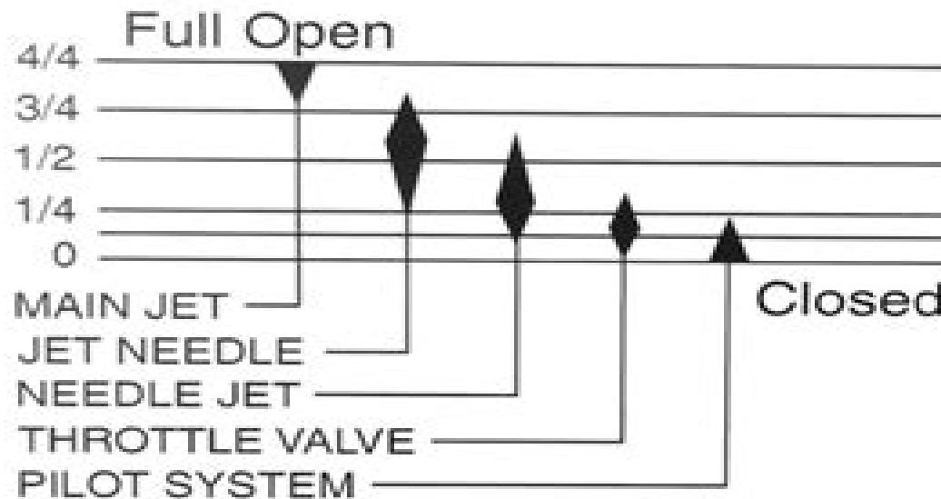
**PILOT SYSTEM includes (PILOT AIR JET, PILOT FUEL JET, PILOT FUEL SCREW)**
