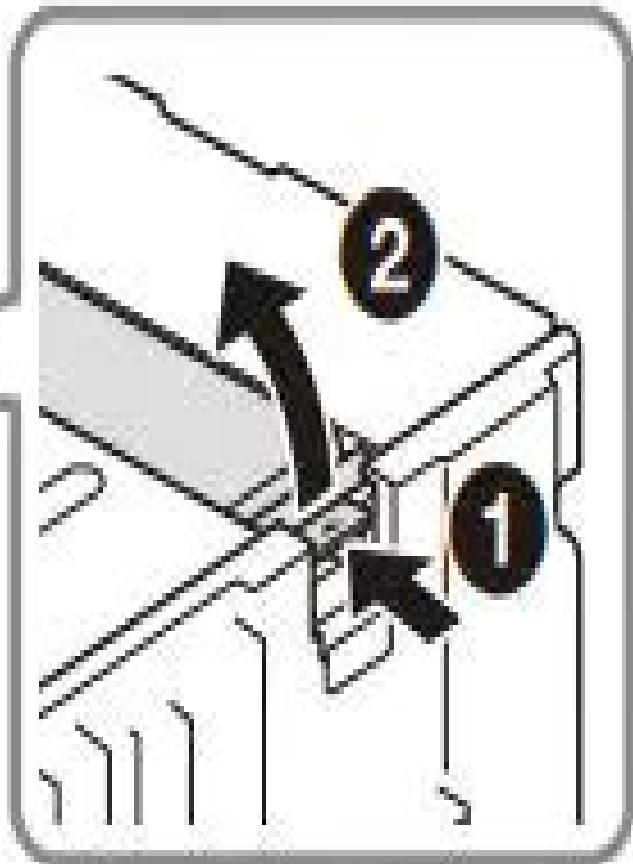
**Release the lock of the cable cover when removing it.**
