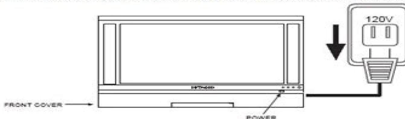
**NOTE:** THE LAMP IS VERY HOT AND MAY CAUSE FIRE OR SEVERE BURNS. WAIT AT LEAST 30-45 MINUTES TO ALLOW THE LAMP TO COOL BEFORE PROCEEDING WITH LAMP REMOVAL.
