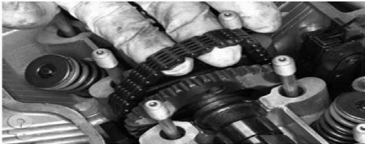
Loop the cam chain over the sprocket.
