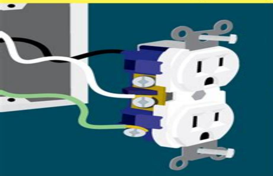
After removing the screws which hold the outlet in place, gently pull it out of the box.
