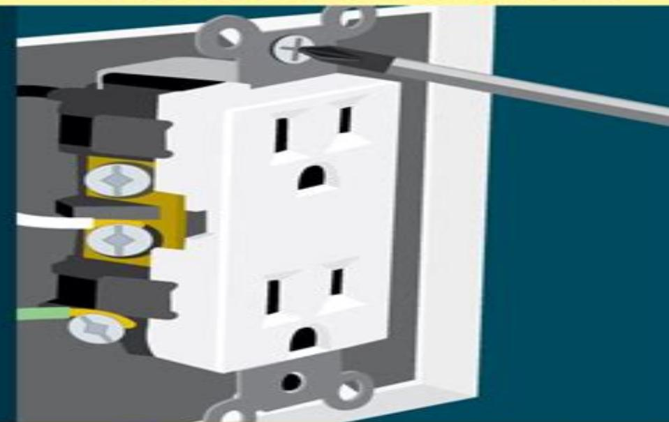
Screw the outlet back into the box with the two Phillips screws.
