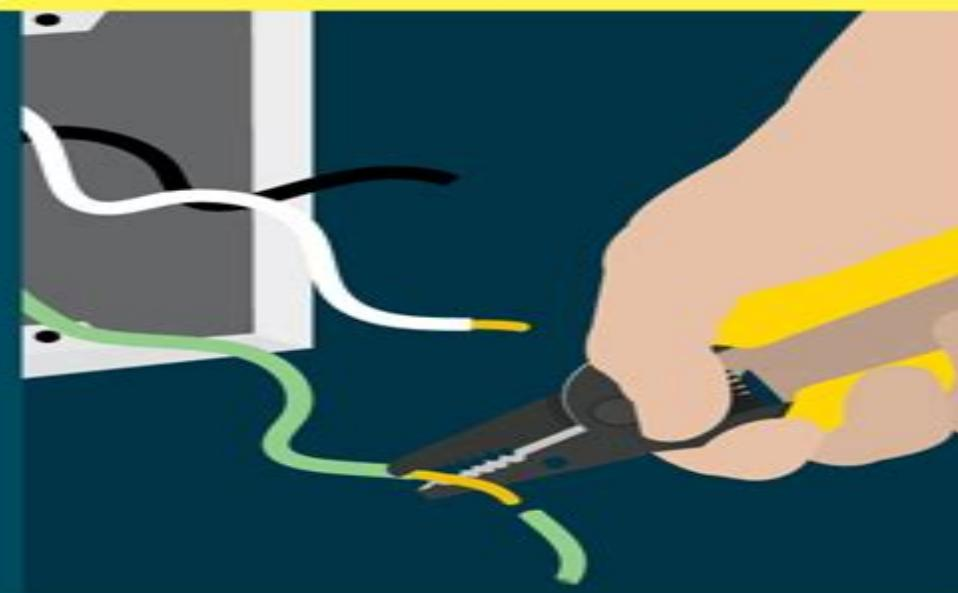
Use your wire strippers to cut back each wire to expose  $1/4"$  to  $1/2"$  of copper wire.
