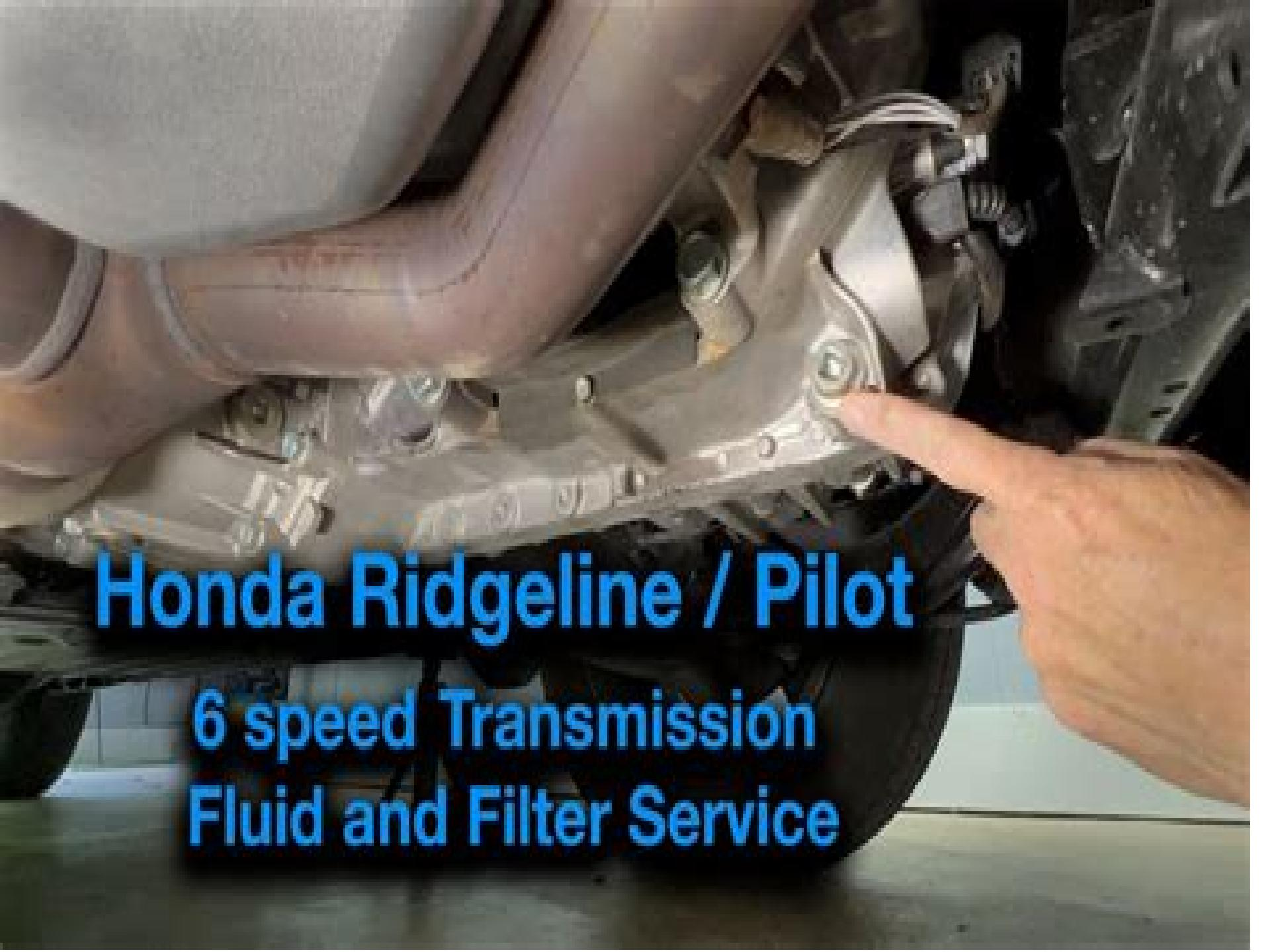
A close-up photograph of the underside of a silver Honda Ridgeline or Pilot. A person's hand is pointing with their index finger towards a circular drain plug on the transmission housing. The transmission is a 6-speed automatic, as indicated by the text in the overlay. The background is dark and metallic.
