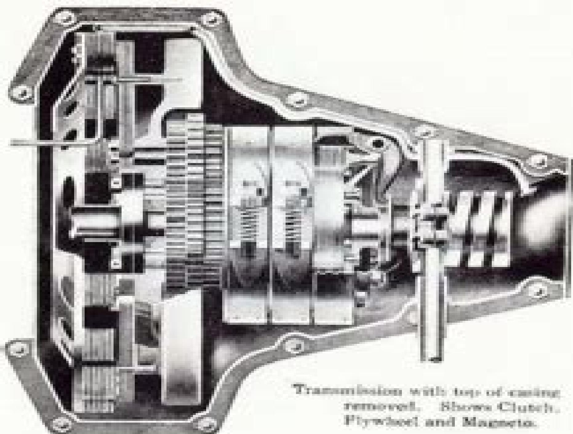
Transmission with top cover removed. Shows Clutch, Flywheel and Magneto.
