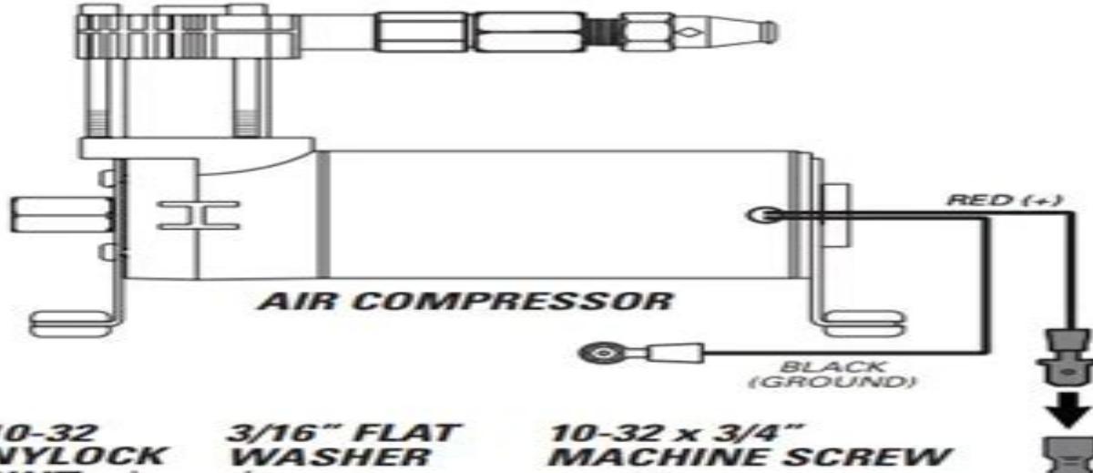
**10-32 NYLOCK NUT**      **3/16" FLAT WASHER**      **10-32 x 3/4" MACHINE SCREW**
