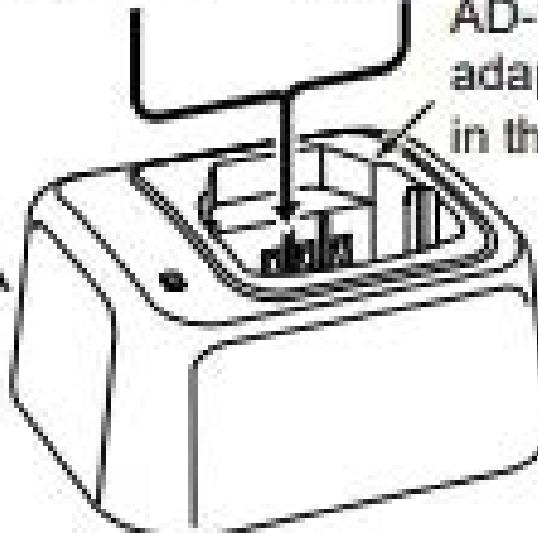
CAUTION: NEVER connect the OPC-515L to a power source using reverse polarity. This will ruin the battery charger.
