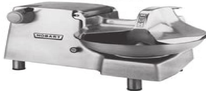
The Model 84186 Food Cutter is designed to cut and mix a wide variety of products. With products in the rotating 18" stainless steel bowl, rotating knives cut and mix them inside the bowl cover. The food cutter is powered by a 1 horsepower motor and is available for single- or three-phase electrical service.
