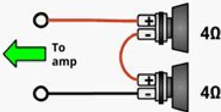
**Series speakers:** The speaker ohm values are added together. Each speaker gets only  $\frac{1}{2}$  of the amp power output.
