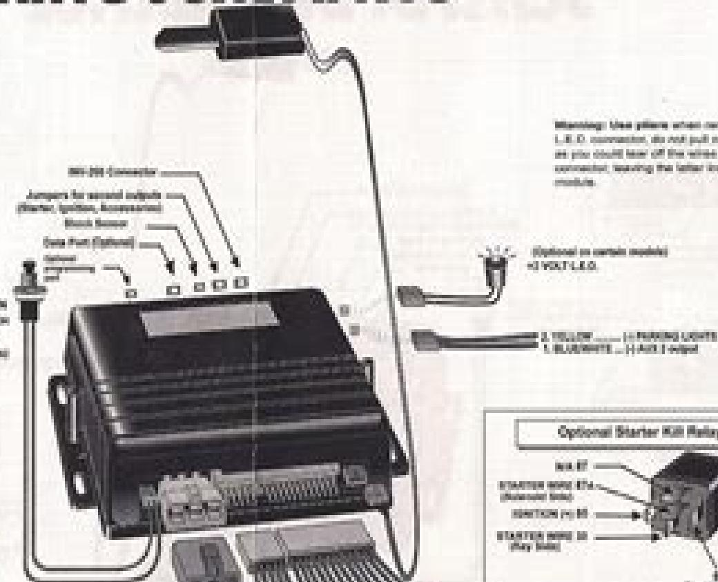
**Warning:** Use gloves when removing the L.E.D. connector, do not pull out the wires as this could tear off the wires from the connector, leaving the latter inside the module.
